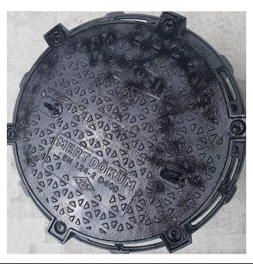
Inspection manhole cover in Spheroidal cast iron EN- GJS-500-7 conforming to norm UNI EN 1563:2004 with load bearing capacity over 400 kN (40 tons), conforming to the load class D400 as set out by norm EN 124:2-2015.
